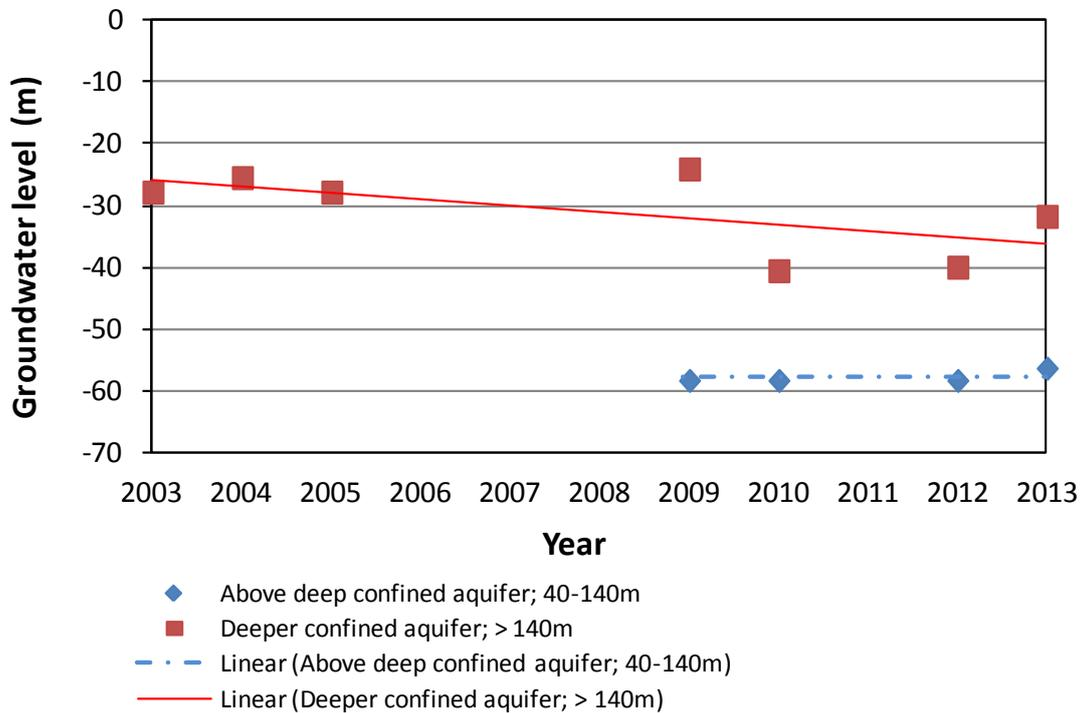
**Figure 4.** Groundwater level trend line of above confined aquifer (40 – 140 m) and deeper confined aquifer (>140m)
